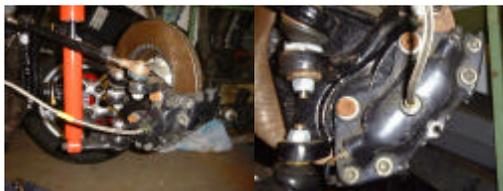
You can use washers or get a piece made for you. You mount the caliper and you will see that the CB spindle has extra material where you can drill a second hole and tap it for M12 as well. You need to spot-face the area for the second hole first to the same level of the original mounting holes and cut off the lower original mounting hole because it will not clear the brake pad and you can not mount the 4pot caliper. Voila...you are done.
