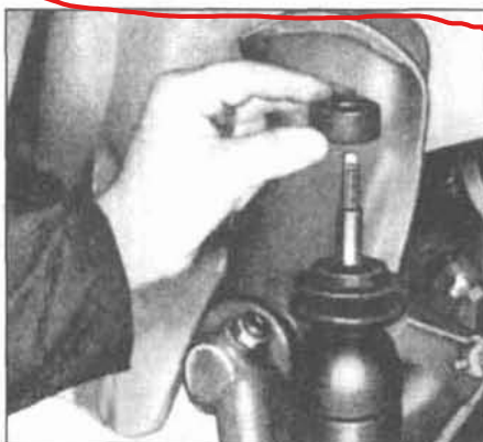
2.12 Install the damping ring on the shock absorber before you slip the damper rod through the upper mounting hole in the shock tower
